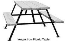
Two heavy duty one piece welded end frames 1-1/4 " X 1-1/4" x 1/8" hot roll angle iron 29-1/2" high x 47-1/2" wide 16-1/2" seat height, end braces are 21-3/4" long. Center brace for flat table top. Dipped in black enamel paint.
