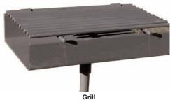
Fire box is made of 3/16" thick steel. Grill connects to post with hex head set screw to prevent wobble & deters theft. 1/2" solid steel bars are only 5/8" apart. Grill flips back yet cannot be removed. Dipped in heat resistant non-toxic black paint. 42" extra long 1-3/8" O.D. thick schedule 40 pipe.19-3/4" wide. 12-1/4" deep, 4-1/2" high. Grill 44 lbs. \$140.10
